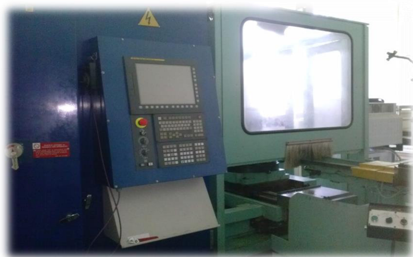
Figure 1.6. The AL 550 Machining Centre
