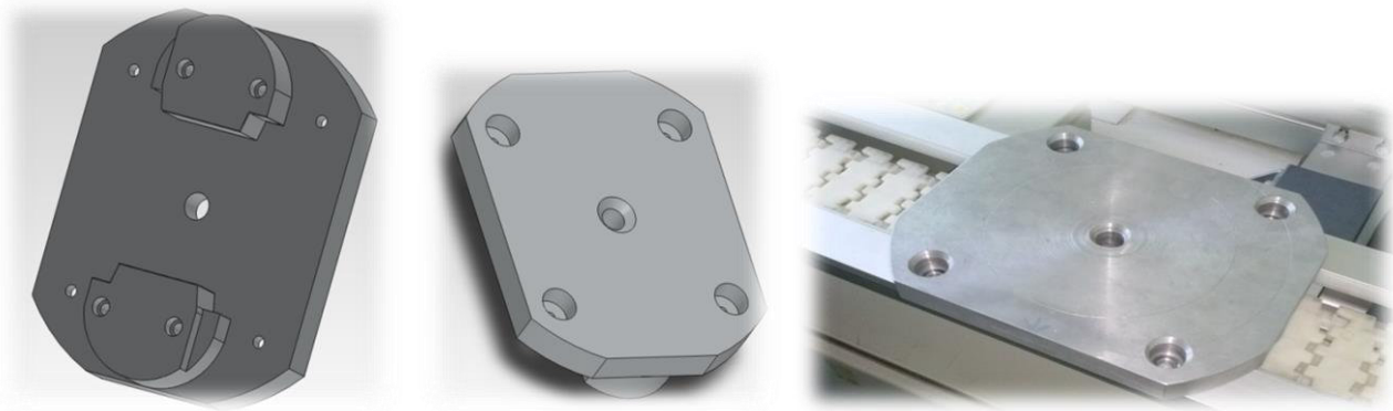
Figure 1.5 The additional transfer pallets
